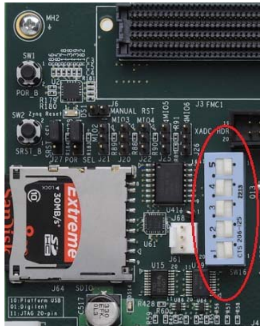
Figure 6-8: Jumper Settings for Booting Linux from SD Card
